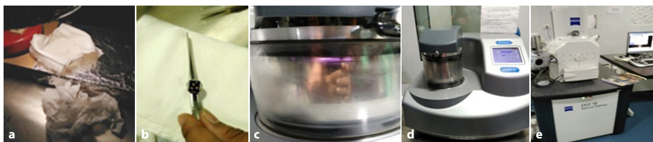
Figure 1 Specimen coating and imaging in scanning electron microscope (Carl Zeiss EVO 18) a – drying; b – mounting and fixing of 2 nd instar nymphs in aluminium stab; c and d – platinum coating in sputter coater; e – imaging in scanning electron microscope
